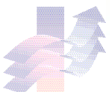
Streak lines showing the separation and recirculation off the suction side of the diffuser blades at the 59% flow condition
