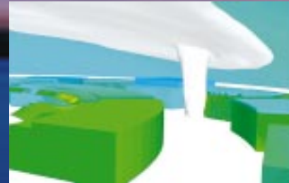
Simulation of a postulated fire in the Dome, showing smoke spread along the roof.
